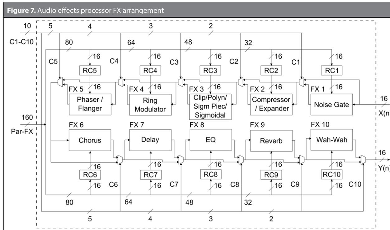
**Figure 8.** Block diagram of effect parameters configuration
