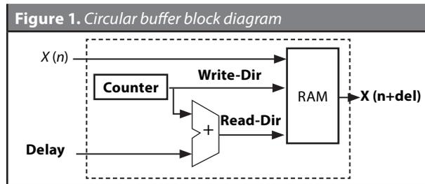
The chorus effect is designed using a circular buffer, an adder, a right-shifter, a low-frequency NCO, and an LFSR (Pérez, 2006) as shown in Figure 2. In a previous study (Liévano, Espinosa & Velasco, 2013), the chorus effect delay is implemented using an LFSR, but in this study the delay is implemented with an NCO given that Pérez (2006) recommends using an LFO.
