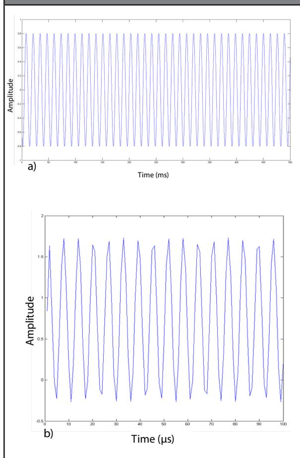
The output signal  $Y_i$  from the audio effect processor is connected to the codec's digital input. The codec's analog output is connected to the audio input of a PC. The analog signal generated by the codec is digitalized by the PC's codec, and this signal is graphed using Matlab. **Figure 14** shows the reverb effect's output signal simulated in Matlab using a sinusoidal signal as input and the processor's output signal  $Y_i$  for the same effect using the audio signal as input.
