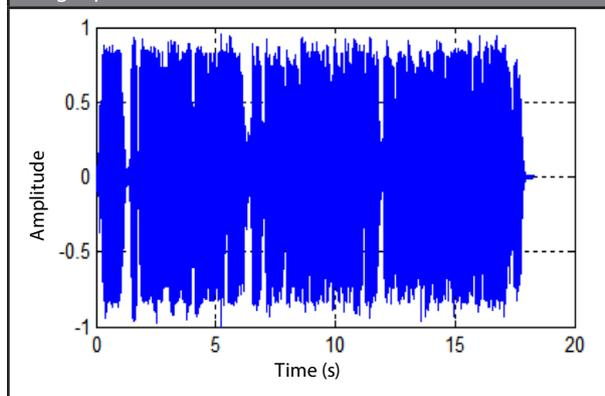
The second processor configuration connects in cascade the compressor, soft clipping, ring modulator, and reverb effects, whose operation parameters are: threshold 0.4 and attenuation 0.6; threshold 0.6; sinusoidal with frequency of 150 Hz; and attenuation 4 and delay 15 ms, respectively. The processor's output signals for the second configuration, using the previous signals, are graphed in Matlab. These are shown in **Figures 19** and **20**, respectively.
