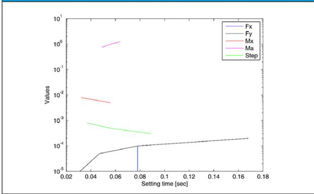
With these values, the control is relatively stable and the response with a tolerance of 1 mm is 0.53 s. If we decrease the tolerance, the setting time increases until it becomes unstable in 1  $\mu\text{m}$  (Figure 11).
