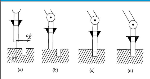
The easiest case for an assembling process is a system with a peg and hole geometry. In this system, a rigid peg is introduced into a rigid hole while the forces are measured by a force sensor, which is placed in the gripper of the assembling robot. With this model, it is possible to analyze all reaction forces between the piece and the environment and to generate a force control. There is a lot of literature about peg-hole systems that supports the research in this article [5].
